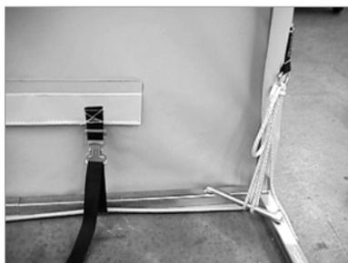
Run the end of the rope around the ½" corner rod, then up through the "D" ring, back around rod and back through the "D" ring. At this point, you can use the "pulley action" to tighten the ropes. Tie off the ends of the ropes.
