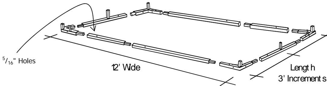
2) Layout the four (4) corners and base pieces and slip fit together. Each base piece has a  $\frac{5}{16}$ " drilled through it. These holes are used to anchor the building to a platform (use  $\frac{1}{4}$ " lag screws – not included) or to the ground (use nail spikes – not included). Do not anchor the base frame at this time, because the fabric cover and web straps are drawn under the frame.
