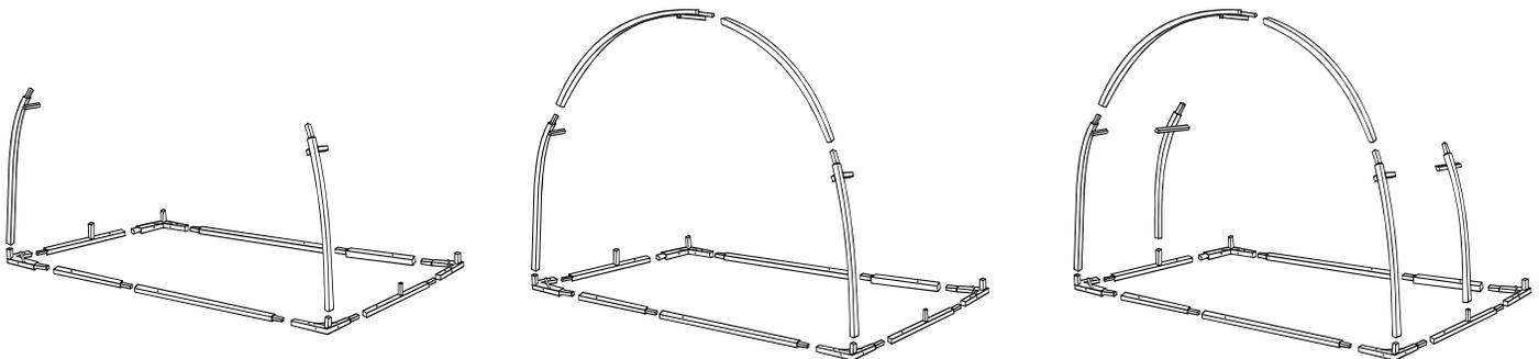
3) Starting at one end of the base (front or back) install the wall legs, then, the arches – one section at a time. (If you put all the wall legs in first, they tend to torque and stress the base frame)
